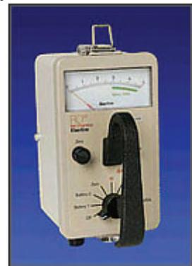
**Figure 3. Ion Chamber**
