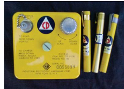
**Figure 9. Direct Reading Pocket Dosimeter**
